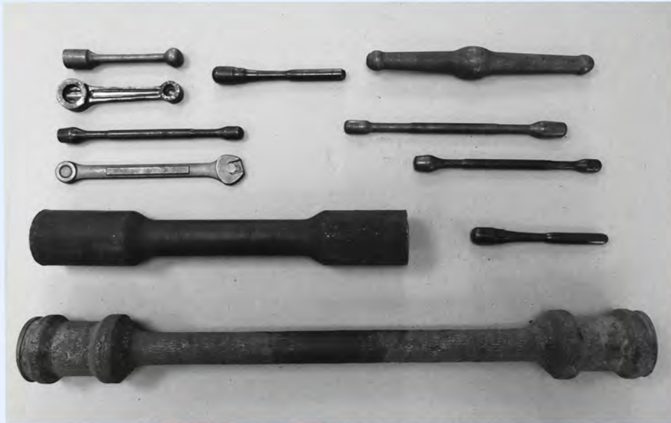
ROLLING PREFORMS FOR SUBSEQUENT STAMPING
