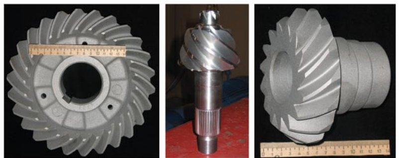
Fig. 1: Complex gear-like components that used to be difficult to harden by conventional induction hardening. In the past all of these parts used to be carburized, but not any more.
