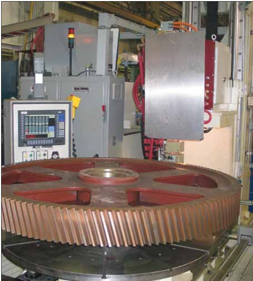
Tooth-by-tooth induction hardening is often used for larger gears. Modern machines are equipped with sophisticated controls and software, allowing precise control over the hardness pattern and tooth-by-tooth documentation for quality control (courtesy Ajax Tocco Magnethermic).
