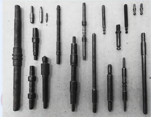
PREFORMS BODIES OF REVOLUTION PRODUCED BY WARM ROLLING
